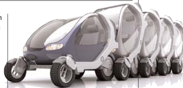
The MIT Smart Cities research team’s drive-by-wire, stackable car
