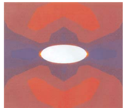
Above: As left, except the hole is formed with the fibres going round it. Strain is much more evenly distributed and the danger spots have gone. This is safe.
